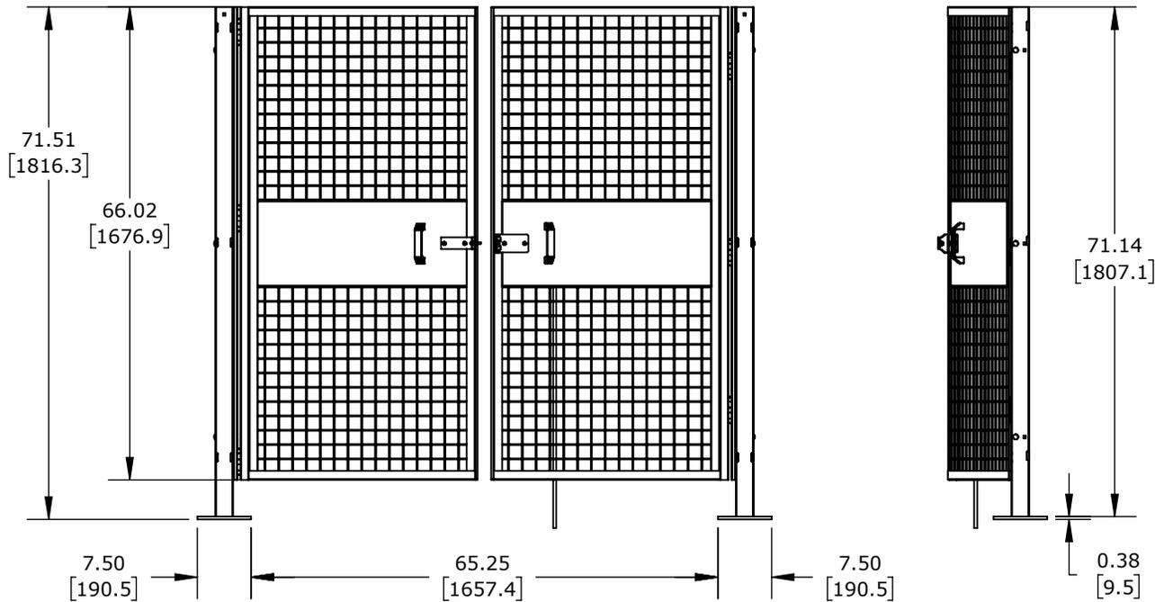
HUSKY RACK AND WIRE VELOX SERIES MACHINE GUARDING DOOR, DOUBLE SWING, 72 X 72IN, 2 X 2IN GRID, CARBON STEEL, YELLOW AND BLACK. 2 DOOR POSTS XG5506D AND MOUNTING HARDWARE INCLUDED.
