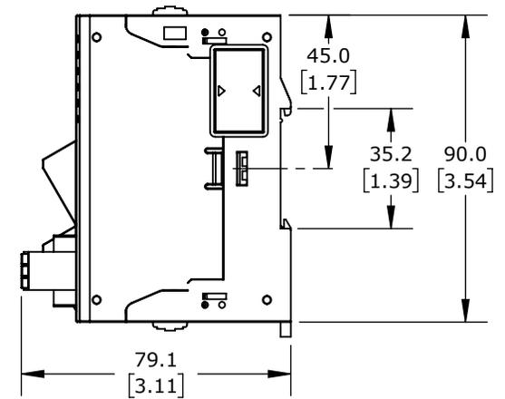
LS ELECTRIC XMC PROGRAMMABLE MOTION CONTROLLER, MICROSD CARD SLOT, ETHERNET AND USB B PORTS, ETHERCAT MASTER AND MODBUS TCP, UP TO (16) AXES AND UP TO (18) VIRTUAL AXES, EXTERNAL 24 VDC REQUIRED, OPTIONAL XEL-BSSCT BUS COUPLER FOR I/O EXPANSION WITH XGB MODULES
