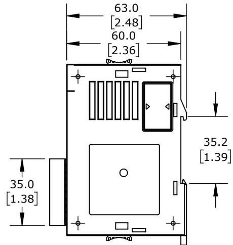
LS ELECTRIC XGB SERIES DISCRETE INPUT MODULE, 8-POINT, 120 VAC, 1 COMMON(S), 8 POINT(S) PER COMMON, REMOVABLE TERMINAL BLOCKS INCLUDED
