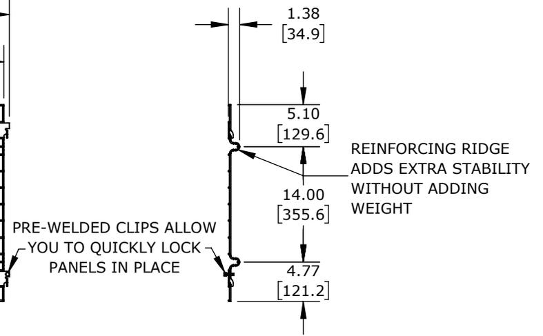
HUSKY RACK AND WIRE VELOX SERIES MACHINE GUARDING PANEL, 24 X 82IN, 2 X 2IN GRID, 8 GAUGE WIRE, CARBON STEEL, BLACK.
