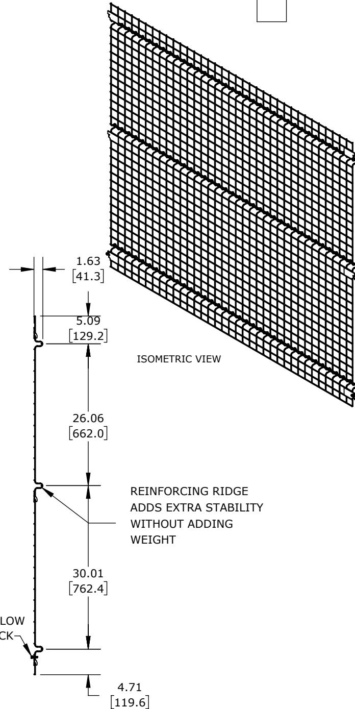
HUSKY RACK AND WIRE VELOX SERIES MACHINE GUARDING PANEL, 66 X 70IN, 2 X 2IN GRID, 8 GAUGE WIRE,
