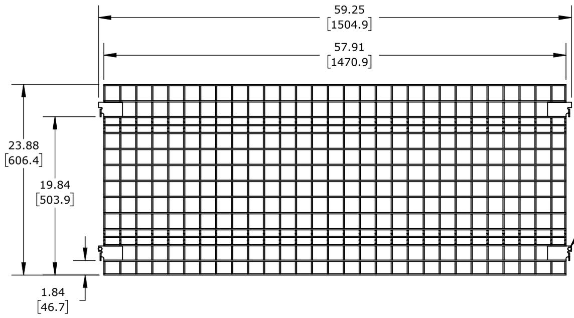
PRE-WELDED CLIPS ALLOW YOU TO QUICKLY LOCK PANELS IN PLACE
