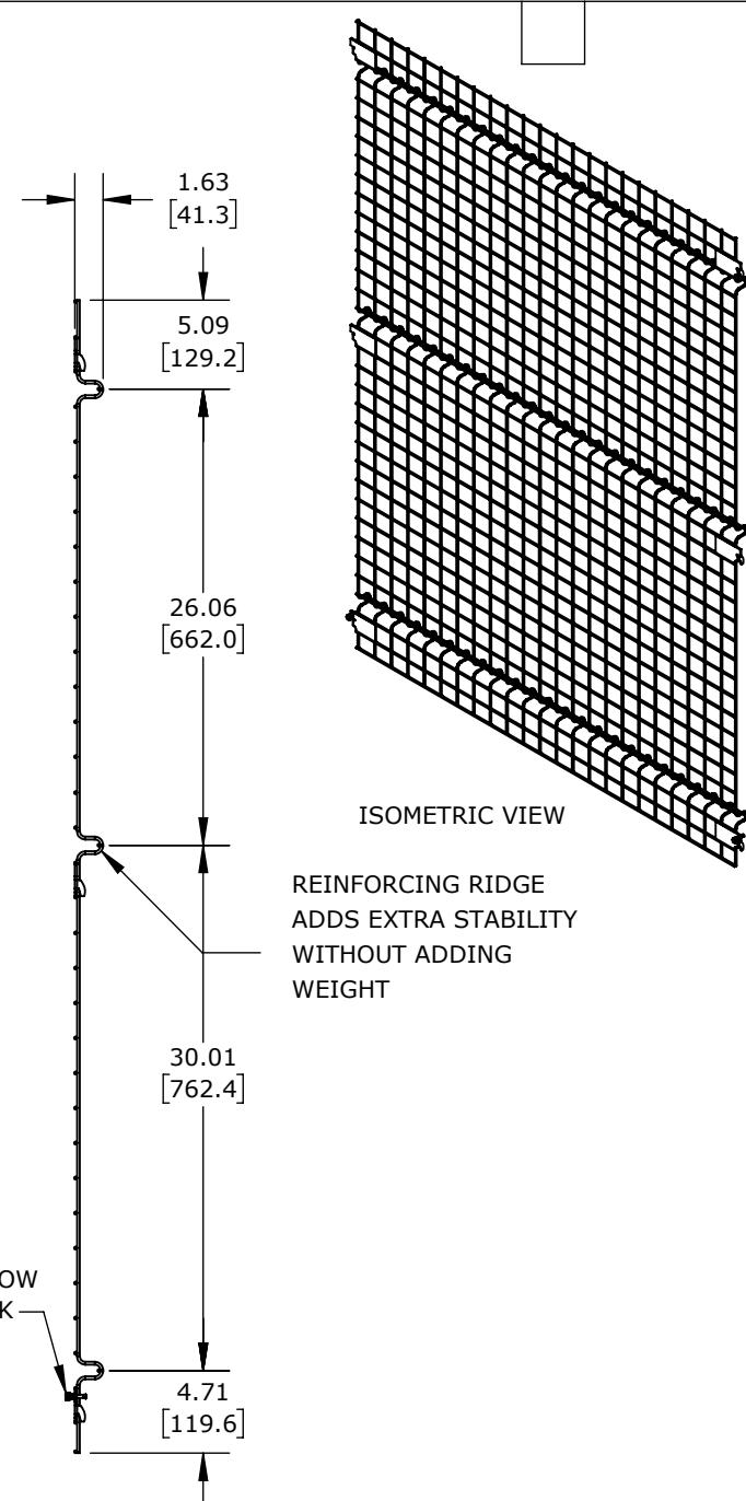
HUSKY RACK AND WIRE VELOX SERIES MACHINE GUARDING PANEL, 66 X 46IN, 2 X 2IN GRID, 8 GAUGE WIRE,
