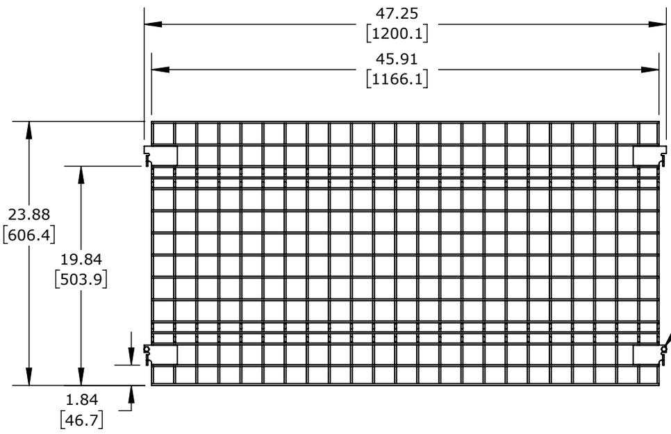
PRE-WELDED CLIPS ALLOW YOU TO QUICKLY LOCK PANELS IN PLACE
