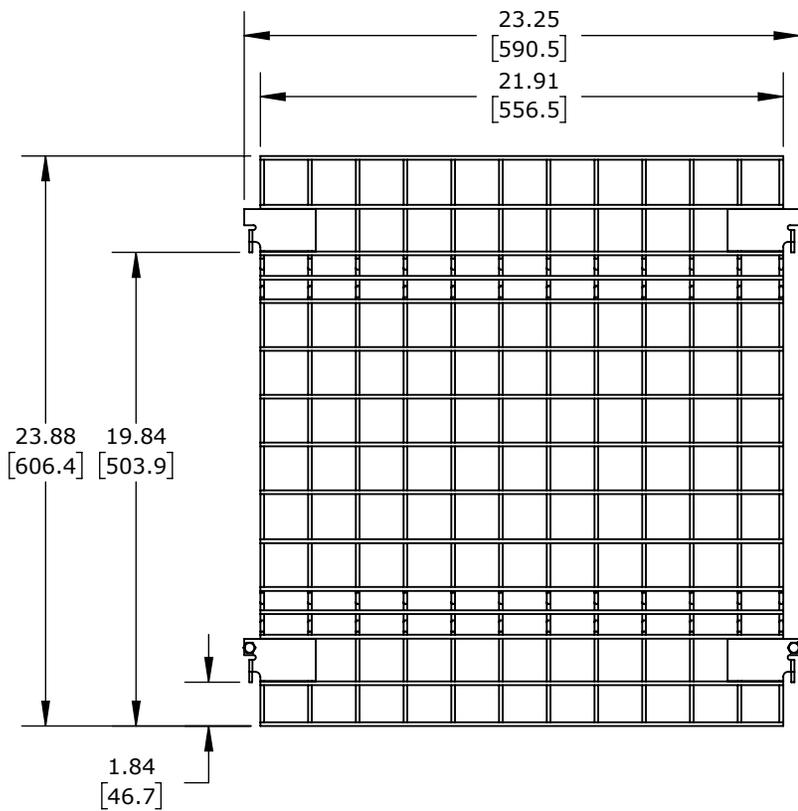
PRE-WELDED CLIPS ALLOW YOU TO QUICKLY LOCK PANELS IN PLACE
