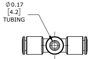
UNION TEE, NICKEL PLATED BRASS BODY, (3) 5/32IN (4MM) PUSH-TO-CONNECT.
