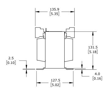
OPEN CORE, 800 VA, 1-PHASE, 208/230/380/400/415/440/460/480/500/525/550/575/600 VAC PRIMARY, 115/230 VAC SECONDARY, 50/60 Hz, PANEL MOUNT.
