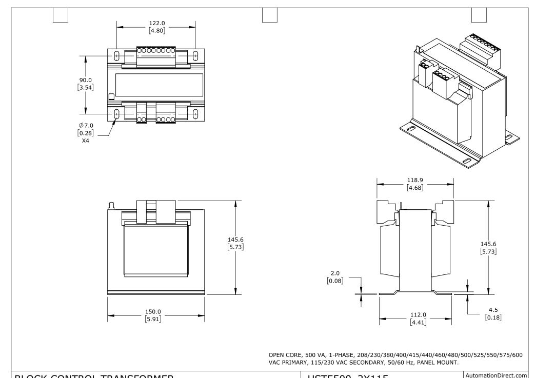
**BLOCK CONTROL TRANSFORMER** USTE500 2X115 1-800-633-0405 PART DIMENSIONS MAY DIFFER SLIGHTLY METRIC UNITS USED UNLESS OTHERWISE 3rd NOT TO mm LATEST VERSION SHEET 1 OF 1 ANGLE [inch] SCALE FOR PART DESIGN SPECIFIED UNITS ARE: 10/31/2024 DUE TO MANUFACTURER'S VARIANCES
