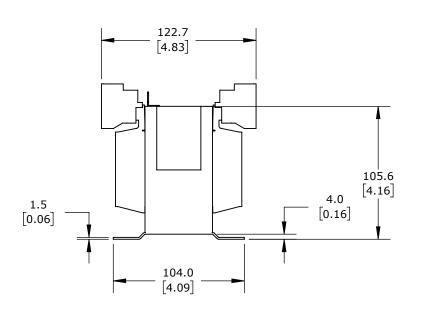
OPEN CORE, 400 VA, 1-PHASE, 208/230/380/400/415/440/460/480/500/525/550/575/600 VAC PRIMARY, 12/24 VAC SECONDARY, 50/60 Hz, PANEL MOUNT.
