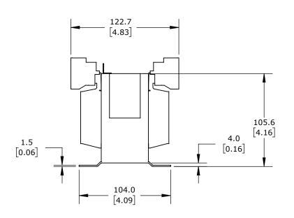
OPEN CORE, 400 VA, 1-PHASE, 208/230/380/400/415/440/460/480/500/525/550/575/600 VAC PRIMARY, 115/230 VAC SECONDARY, 50/60 Hz, PANEL MOUNT.
