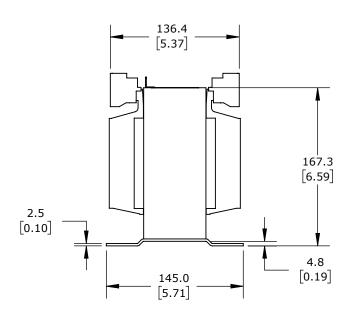
OPEN CORE, 1.6 KVA, 1-PHASE, 208/230/380/400/415/440/460/480/500/525/550/575/600 VAC PRIMARY, 115/230 VAC SECONDARY, 50/60 Hz, PANEL MOUNT.
