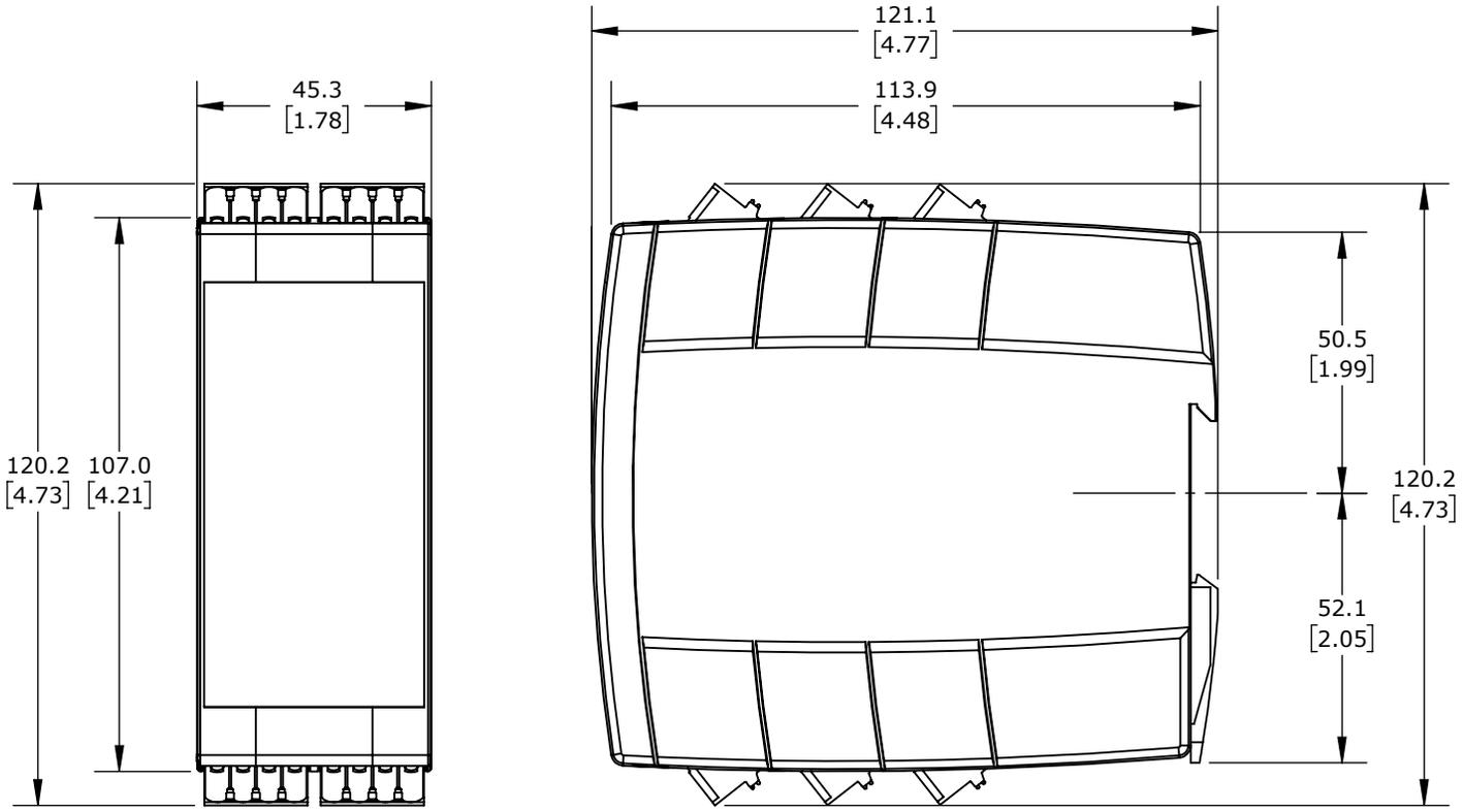
DOLD SAFETY RELAY, MOTOR STANDSTILL, SPEED AND SAFETY GATE MONITORING, MULTI DELAY FUNCTIONS, (2) NAMUR SENSOR INPUTS AND/OR (1) ENCODER, 2-CHANNEL, 24 VDC, (4) N.O. SAFETY OUTPUT(S), (2) STATUS MONITORING OUTPUT(S), PUSH-IN CAGE CLAMP.
