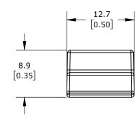
1 HOLE. FOR USE WITH PBC UGT040-XXXX GUIDE TRACKS.
