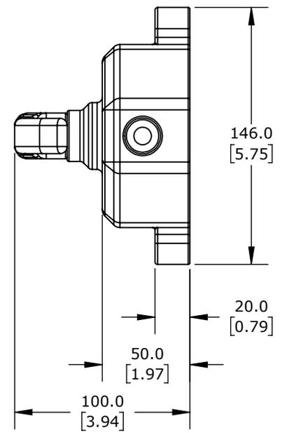
IDEM HANDLE AND MOUNTING PLATE, ROTARY, RIGHT HAND. FOR USE WITH UGB SERIES 4-STATION UNIVERSAL GATE BOXES.
