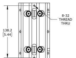
CAM FOLLOWER BEARING, 6IN OVERALL LENGTH, STEEL, 1IN INSIDE DIAMETER, ALUMINUM HOUSING, ADJUSTABLE RUNNING CLEARANCE. FOR USE WITH 1IN DIAMETER PBC SHAFTS.
