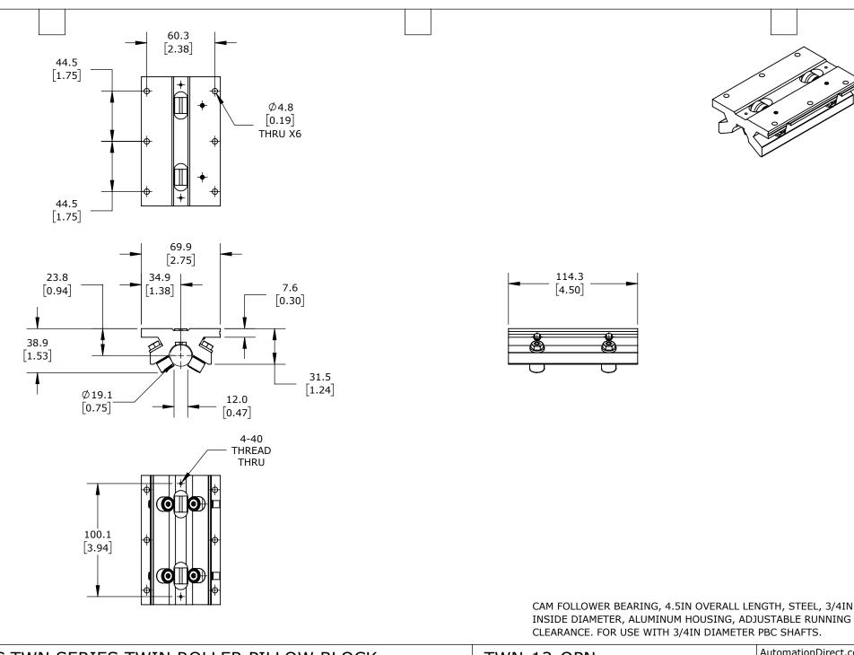
AutomationDirect.com PBC TWN SERIES TWIN ROLLER PILLOW BLOCK TWN-12-OPN 1-800-633-0405 PART DIMENSIONS MAY DIFFER SLIGHTLY NOT TO METRIC UNITS USED UNLESS OTHERWISE LATEST VERSION 3rd mm SHEET 1 OF 1 **ANGLE** SCALE FOR PART DESIGN [inch] DUE TO MANUFACTURER'S VARIANCES SPECIFIED UNITS ARE: 1/13/2025
