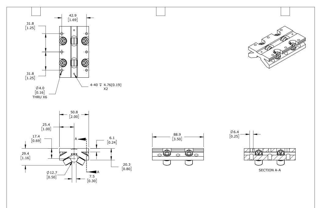
CAM FOLLOWER BEARING, 3.5IN OVERALL LENGTH, STEEL, 1/2IN INSIDE DIAMETER, ALUMINUM HOUSING, ADJUSTABLE RUNNING CLEARANCE. FOR USE WITH 1/2IN DIAMETER PBC SHAFTS.
