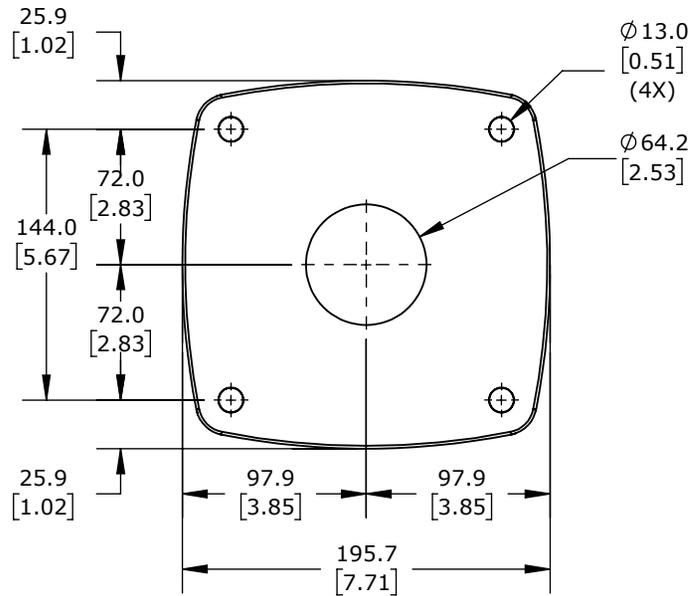
TEKNOKOL SUSPENSION ARM FITTING, RIGHT-ANGLE TOP-MOUNT SWIVEL BASE, 310 DEGREES MOVEMENT RANGE, ALUMINUM, RAL 7035 LIGHT GRAY. FOR USE WITH TK120 SUSPENSION ARM PROFILE.
