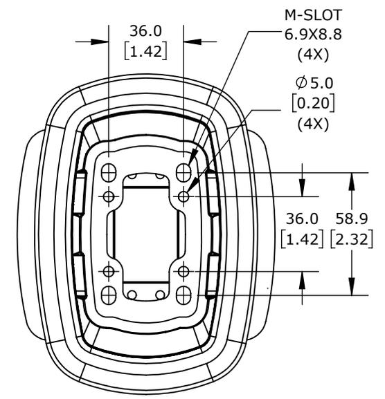
TEKNOKOL SUSPENSION ARM FITTING, STRAIGHT WALL-MOUNT SWING BASE, PLUS OR MINUS 90 DEGREES HORIZONTAL MOVEMENT RANGE, CARBON STEEL, RAL 7035 LIGHT GRAY. FOR USE WITH TK060 SUSPENSION ARM PROFILE.
