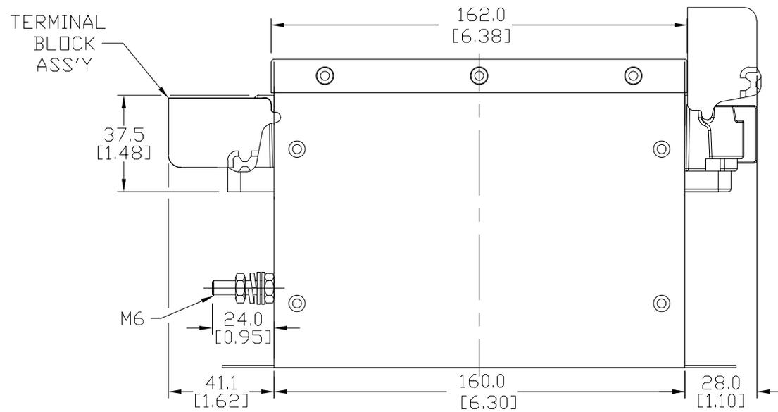
LS ELECTRIC EMI INPUT FILTER 550 VAC, 3-PHASE, 60A, PANEL MOUNT, EMI/RFI FILTERING, DRIVE RATED, STANDARD PERFORMANCE, SCREW TERMINALS, FOR USE WITH 1-PHASE OR 3-PHASE AC DRIVES
