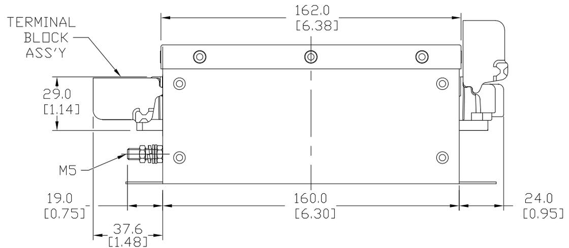
LS ELECTRIC EMI INPUT FILTER 550 VAC, 3-PHASE, 40A, PANEL MOUNT, EMI/RFI FILTERING, DRIVE RATED, STANDARD PERFORMANCE, SCREW TERMINALS, FOR USE WITH 1-PHASE OR 3-PHASE AC DRIVES
