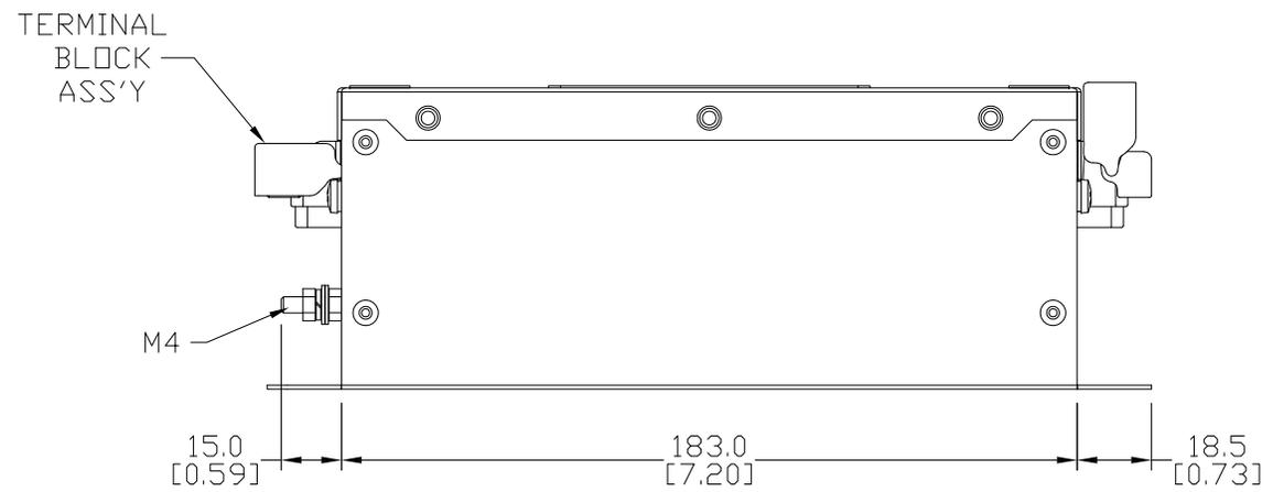
LS ELECTRIC EMI INPUT FILTER 550 VAC, 3-PHASE, 30A, PANEL MOUNT, EMI/RFI FILTERING, DRIVE RATED, STANDARD PERFORMANCE, SCREW TERMINALS, FOR USE WITH 1-PHASE OR 3-PHASE AC DRIVES
