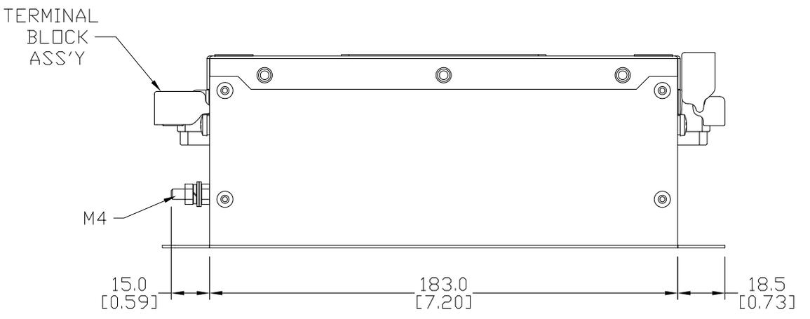
LS ELECTRIC EMI INPUT FILTER 550 VAC, 3-PHASE, 20A, PANEL MOUNT, EMI/RFI FILTERING, DRIVE RATED, STANDARD PERFORMANCE, SCREW TERMINALS, FOR USE WITH 1-PHASE OR 3-PHASE AC DRIVES
