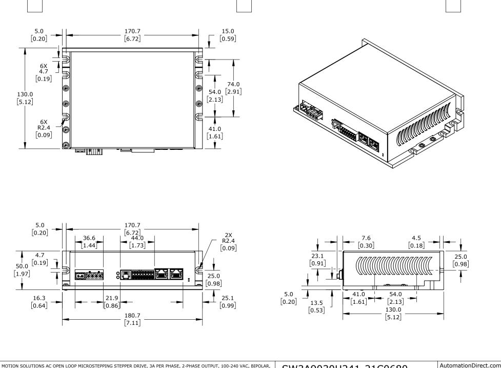
EVER MOTION SOLUTIONS AC OPEN LOOP MICROSTEPPING STEPPER DRIVE, 3A PER PHASE, 2-PHASE OUTPUT, 100-240 VAC, BIPOLAR, VELOCITY AND POSITION MODE, 200 TO 65536 STEPS PER REVOLUTION, (2) ETHERNET 100BASE-TX (RJ45) AND (1) RJ11 PORT(s)
