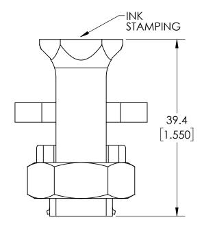
COPPER SPLIT BOLT CONNECTOR FOR 2 CONDUCTORS
