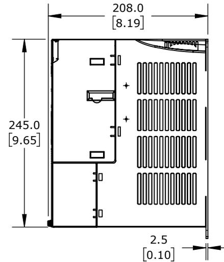
SureServo2 SERVO DRIVE, 2 kW, 460 VAC, 3-PH, 1 RS-485 RJ45 PORT(S), MODBUS, FOR USE WITH 2 kW SYSTEMS, OPTIONAL Ethernet/IP & MODBUS TCP CARDS AVAILABLE
