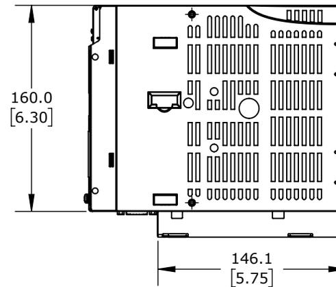
SureServo2 SERVO DRIVE, 750W, 460 VAC, 3-PH, 1 RS-485 RJ45 PORT(S), MODBUS, FOR USE WITH 750W SYSTEMS, OPTIONAL Ethernet/IP & MODBUS TCP CARDS AVAILABLE
