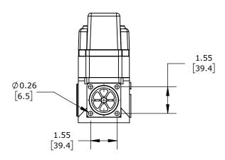
2-WAY, 2-POSITION, GLASS-FILLED NYLON BODY, STACKABLE, 120 VAC OPERATING VOLTAGE, 12VA, 18MM DIN STYLE WIRING PLUG. RA-3903 HIGH-FLOW TURBINE AND SF-9130 SCREEN INCLUDED.
