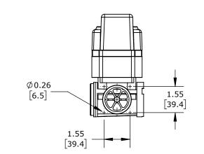
2-WAY, 2-POSITION, GLASS-FILLED NYLON BODY, STACKABLE, 24 VAC/VDC OPERATING VOLTAGE, 7.2W, 18MM DIN STYLE WIRING PLUG. RA-3903 HIGH-FLOW TURBINE AND SF-9130 SCREEN INCLUDED.
