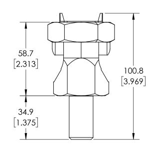
COPPER SPLIT BOLT CONNECTOR FOR 2 CONDUCTORS
