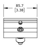
CAM FOLLOWER BEARING, 3.37IN OVERALL LENGTH, STEEL, 1-1/4IN INSIDE DIAMETER, ALUMINUM HOUSING, ADJUSTABLE RUNNING CLEARANCE. FOR USE WITH 1-1/4IN DIAMETER PBC SHAFTS.
