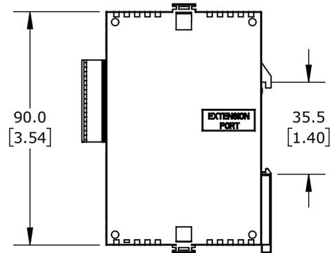
SOLO MODULAR TEMPERATURE CONTROLLER EXTENSION, CURRENT, VOLTAGE, THERMOCOUPLE OR RTD INPUT, 0-10 VDC, 3A SPST RELAY OUTPUT, 24VDC OPERATING VOLTAGE, RS-485
