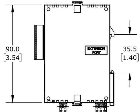
SOLO MODULAR TEMPERATURE CONTROLLER MAIN, CURRENT, VOLTAGE, THERMOCOUPLE OR RTD INPUT, (2) 3A SPST RELAY OUTPUT, 24VDC OPERATING VOLTAGE, RS-485
