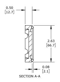
FOR USE WITH CITO STACKFLOW VALVES BODY INLET. BK-9100 BOLT KIT INCLUDED.
