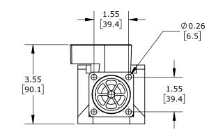
2-WAY, 2-POSITION, GLASS-FILLED NYLON BODY, STACKABLE. FT-200 TEMPERATURE GAUGE AND RA-3903 HIGH-FLOW TURBINE INCLUDED.
