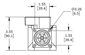
2-WAY, 2-POSITION, GLASS-FILLED NYLON BODY, STACKABLE. RA-3903 HIGH-FLOW TURBINE INCLUDED.
