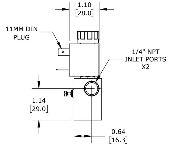
(4) STATIONS, 2-PORT (2-WAY), N.C., 1/4IN FEMALE NPT INLET(s), 1/4IN FEMALE NPT OUTLET(s), CV=0.14, INDIVIDUAL METERING, STAINLESS STEEL BODY, 24 VAC, 6.5 VA, 11mm DIN STYLE WIRING PLUG
