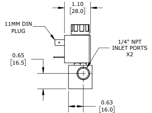
(4) STATIONS, 2-PORT (2-WAY), N.C., 1/4IN FEMALE NPT INLET(s), 1/4IN FEMALE NPT OUTLET(s), CV=0.14, BRASS BODY, 24 VAC, 6.5 VA, 11mm DIN STYLE WIRING PLUG.
