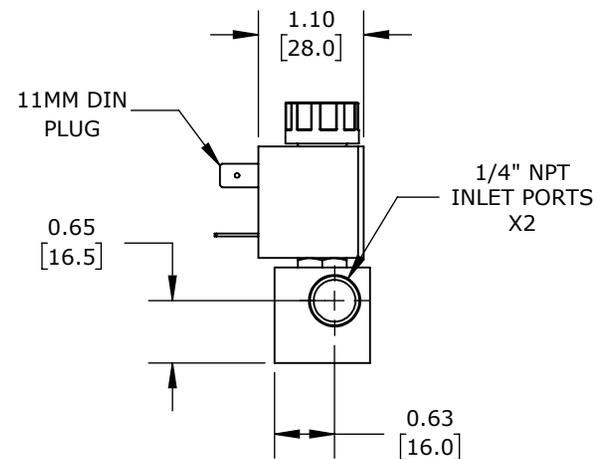
(4) STATIONS, 2-PORT (2-WAY), N.C., 1/4IN FEMALE NPT INLET(s), 1/4IN FEMALE NPT OUTLET(s), CV=0.14, BRASS BODY, 120 VAC, 6.5 VA, 11mm DIN STYLE WIRING PLUG
