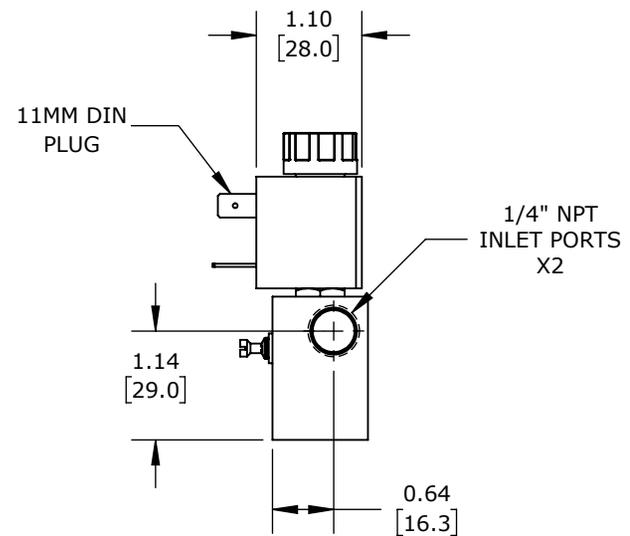
(3) STATIONS, 2-PORT (2-WAY), N.C., 1/4IN FEMALE NPT INLET(S), 1/4IN FEMALE NPT OUTLET(S), CV=0.14, INDIVIDUAL METERING, STAINLESS STEEL BODY, 24 VAC, 6.5 VA, 11mm DIN STYLE WIRING PLUG
