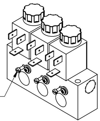
NOTE: FLATHEAD SCREWS FOR METERING FLOW. PHILIPS SCREW AND WASHER FOR LIMITING TRAVEL ON METERING SCREW
