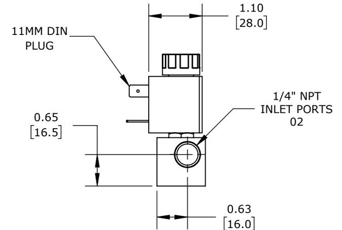
(3) STATIONS, 2-PORT (2-WAY), N.C., 1/4IN FEMALE NPT INLET(s), 1/4IN FEMALE NPT OUTLET(s), CV=0.14, STAINLESS STEEL BODY, 24 VAC, 6.5 VA, 11mm DIN STYLE WIRING PLUG
