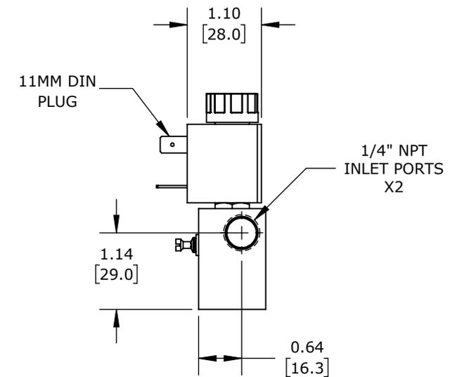
(3) STATIONS, 2-PORT (2-WAY), N.C., 1/4IN FEMALE NPT INLET(s), 1/4IN FEMALE NPT OUTLET(s), CV=0.14, INDIVIDUAL METERING, BRASS BODY, 24 VAC, 6.5 VA, 11mm DIN STYLE WIRING PLUG
