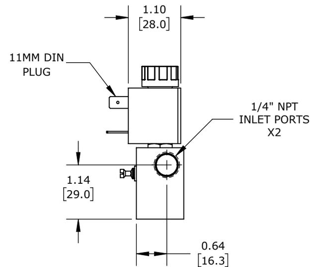
(3) STATIONS, 2-PORT (2-WAY), N.C., 1/4IN FEMALE NPT INLET(S), 1/4IN FEMALE NPT OUTLET(S), CV=0.14, INDIVIDUAL METERING, STAINLESS STEEL BODY, 24 VDC, 4W, 11mm DIN STYLE WIRING PLUG
