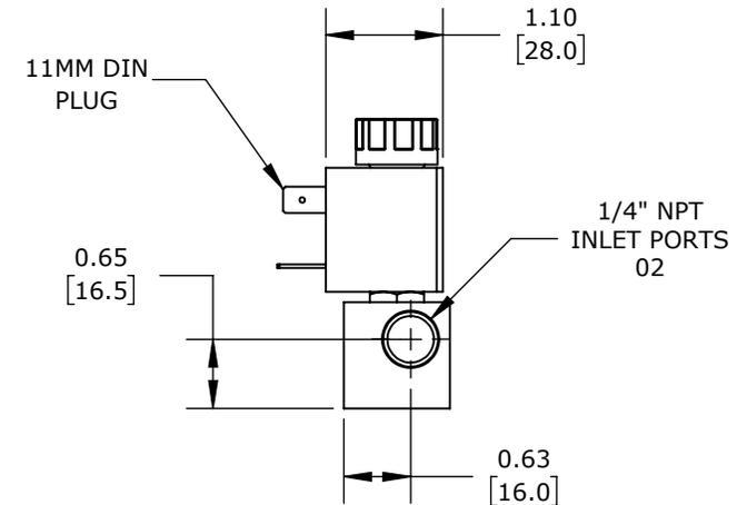
(3) STATIONS, 2-PORT (2-WAY), N.C., 1/4IN FEMALE NPT INLET(s), 1/4IN FEMALE NPT OUTLET(s), CV=0.14, STAINLESS STEEL BODY, 120 VAC, 6.5 VA, 11mm DIN STYLE WIRING PLUG.
