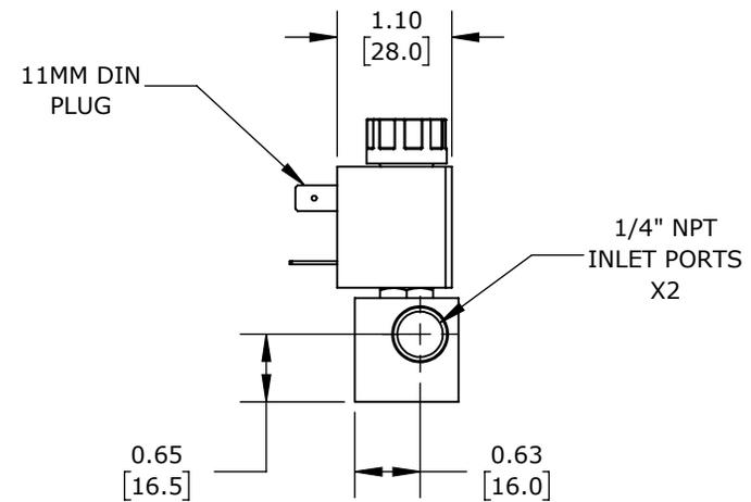
(2) STATIONS, 2-PORT (2-WAY), N.C., 1/4IN FEMALE NPT INLET(s), 1/4IN FEMALE NPT OUTLET(s), CV=0.14, BRASS BODY, 24 VDC, 4W, 11mm DIN STYLE WIRING PLUG
