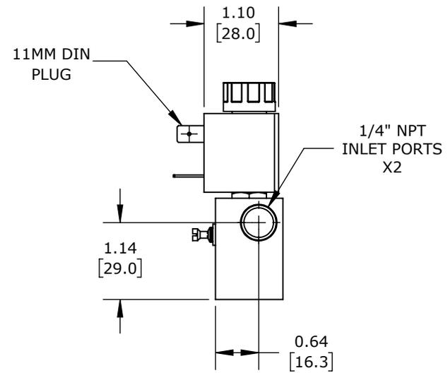
(2) STATIONS, 2-PORT (2-WAY), N.C., 1/4IN FEMALE NPT INLET(s), 1/4IN FEMALE NPT OUTLET(s), CV=0.14, INDIVIDUAL METERING, STAINLESS STEEL BODY, 120 VAC, 6.5 VA, 11mm DIN STYLE WIRING PLUG.
